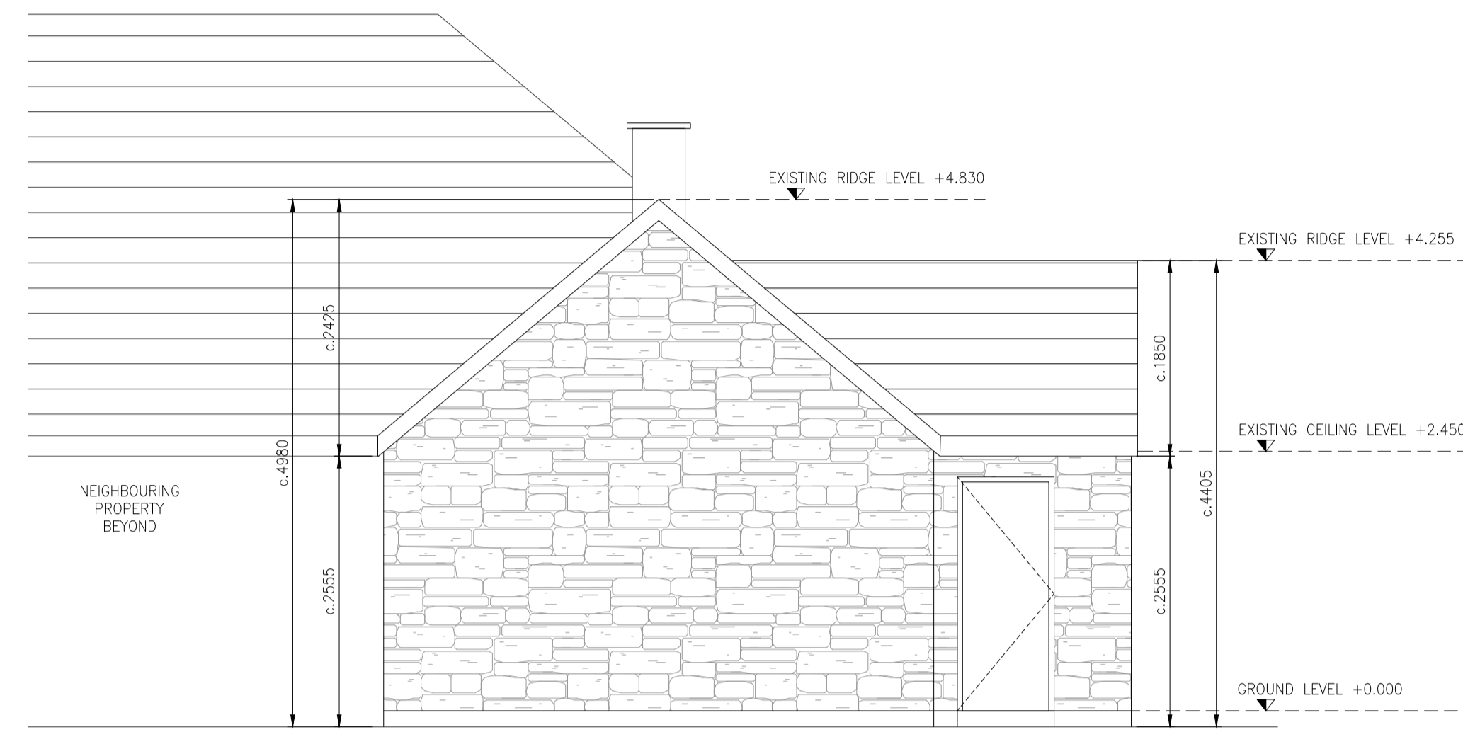
HOUSETYPE B - SOUTH ELEVATION (EXISTING) SCALE 1:50
